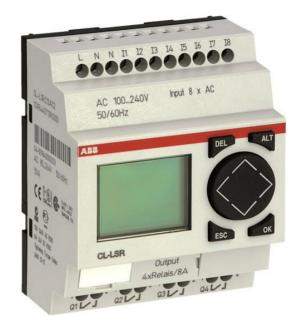
The CL-LSR.12AC2 is a logic relay from the CL range. It has 8 digital inputs and 4 relay outputs. The logic relay operates with an input voltage of 100-240 V AC and is equipped with an onboard display and a keypad. 128 rungs with 3 contacts in series plus 1 coil can be programmed. The following functions are available: 16 freely editable display texts, 16 multifunction timing relays, 4 operating hours counters, 16 analog value comparators and threshold value switches
