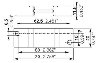
The ADP.01 adapter for screw mounting is an accessory. The adapter allows the screw mounting of a S housing on panel or wall.
