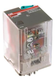
The CR-U048AC3L pluggable interface relay is from the CR-U (universal) relay range. This relay operates with a 48 V AC rated control supply voltage and has 3 c/o (SPDT) output contacts rated at 250 V / 10 A. The relay has an integrated orange test button for manual actuation and locking of the output contacts and an integrated LED. Standard sockets, logic sockets, pluggable function modules, holder and marker are available as accessories.
