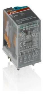
The CR-M048DC2L pluggable interface relay is from the CR-M (miniature) relay range. This relay operates with a 48 V DC rated control supply voltage and has a 2 c/o (SPDT) output with contacts rated at 250 V / 12 A. The relay has an integrated blue test button for manual actuation and locking of the output contacts and an integrated LED. Standard sockets, logic sockets, pluggable function modules, holder and marker are available as accessories.
