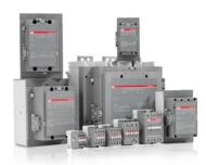
A 3-phase Contactor suitable for Capacitor switching application. Maximum permissible peak current 100 times the nominal RMS current. Operated with a control voltage, versions from 24…….690 V
