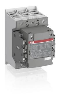
A 3-phase Contactor suitable for various applications such as Motor starting, Isolation, By-pass and Distribution application up to max 690 V. Operated with wide control voltage range 48-130 V, 50/60 Hz and DC
