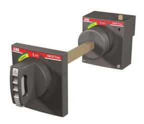
ROTARY HANDLE OPERATING MECHANISM STANDARD ADJUSTABLE DEPTH L=500 MM WITH PADLOCK DEVICE AND DOOR INTERLOCK FOR WITHDRAWABLE CIRCUIT-BREAKER XT2-XT4
