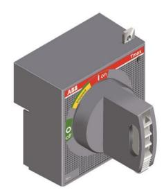
ROTARY HANDLE OPERATING MECHANISM EMERGENCY ADJUSTABLE DEPTH L=500 MM WITH PADLOCK DEVICE AND DOOR INTERLOCK FOR C.BREAKER WITHDRAWABLE T6
