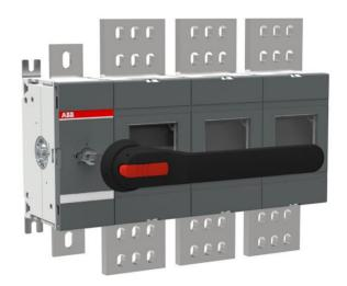
Including terminal bolt kit, a black ON-OFF plastic handle OHB200J12P and shaft OXP12x280 as standard. The handle is IP65 protected, padlockable in the OFF-position and with door interlock in the ON-position. The shaft is adjustable for a range of installation depths.
