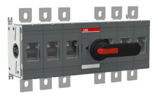
Including terminal bolt kit, a black ON-OFF plastic handle and shaft as standard. The handle is IP65 protected, padlockable in the OFF position and with door interlock in the ON-position. The shaft is adjustable for a depth of installation ranges.
