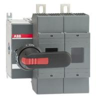
Including terminal bolt kit, a black ON-OFF plastic handle and shaft as standard. The handle is IP65, NEMA 1, 3R, 12 protected, padlockable in the OFF-position and with door interlock in the ON-position. The shaft is adjustable for a range of installation depths. Fuse standards UL 248.
