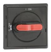
Selector type handle. Indication I-O and ON-OFF. No separate shaft needed. Padlockable with max. 3 padlocks, IP 65, hole distance 36/48 mm, NEMA 1, 3R, 12, black, OT16...125FT
