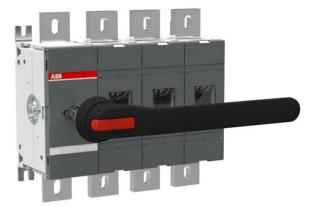
Including a black ON-OFF plastic handle and shaft as standard. The handle is IP65 protected,padlockable in the OFF-position and with door interlock in the ON-position. The shaft is adjustable for arange of installation depths.
