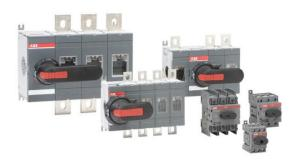
Including a black ON-OFF plastic handle and shaft as standard. The handle is IP65 protected, padlockable in the OFF-position and with door interlock in the ON-position. The shaft is adjustable for a range of installation depths.
