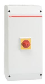
EMC safety switch 3-p.400V AC23A 45kW AC22A A Plastic enclosure IP65 Yellow-red Selector handle
