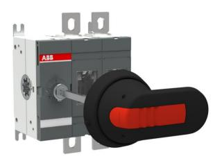
Including terminal bolt kit, a black ON-OFF plastic handle and shaft as standard. The handle is IP65 protected, padlockable in the OFF-position and with door interlock in the ON-position. The shaft is adjustable for a range of installation depths.
