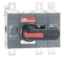
Including a black ON-OFF plastic handle and shaft as standard. The handle is IP65 protected,padlockable in the OFF-position and with door interlock in the ON-position. The shaft is adjustable for arange of installation depths.
