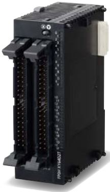
Input 32 points DC Transistor output (sink) 32 points AFP0HXY64D2T
