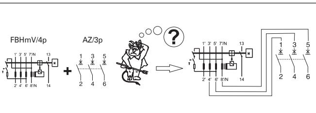
**Mounting arrangement residual current protection unit - shunt trip release - miniature circuit breaker - auxiliary contact**
