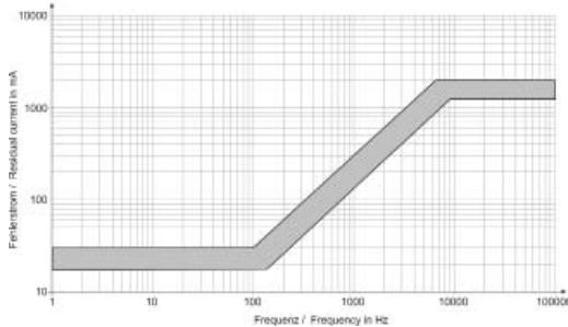
Tripping current frequency response 100 mA Type B
