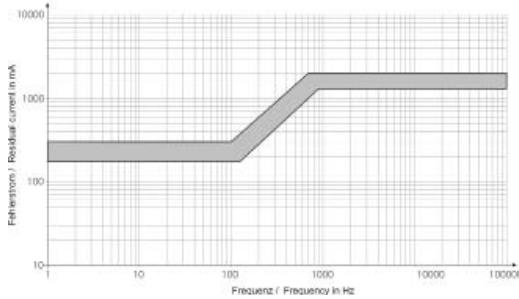
Tripping current frequency response 500 mA Type S/Bfq
