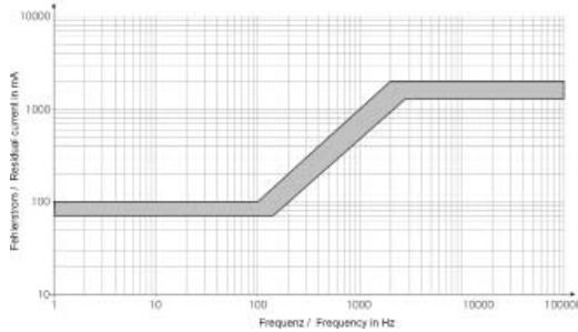
Tripping current frequency response 300 mA Type S/Bfq
