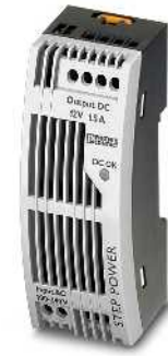
Stromversorgung, 1 AC, 12 V DC, 1.5 A flache Bauform, NEC Class 2
