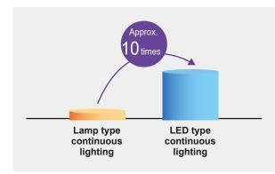
The LED type features extremely long light-source life span compared to the lamp type. As compared to the estimated lamp life span of 1,500 hours <sup>(Note 1)</sup>, the estimated LED life span is 15,000 hours <sup>(Note 2)</sup>.
