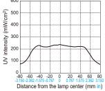
Lamp: Metal halide lamp (1.5 kW) Reflector: DICOOL optical mirror Distance: 130 mm 5.118 in
