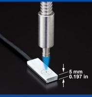
The UV intensity can be relative measured (Note 1) at the actual position by using the slim UV sensor. It can also automatically adjust the UV intensity to the preset level. Since the sensor only has 5 mm (0.197 in) thickness, which is similar to the workpiece, the intensity measurement is possible without removing the system from the production line, facilitating
