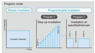
The irradiation can be programmed to controls the irradiation power and time depending on the resin and curing appication, supporting high-quality and high-precision bonding with minimum cure shrinkage. In addition to the simple irradiation mode which irradiation is continuously performed at a constant intensity, up to 10 steps 7 different irradiation patterns (7 product types) can be programmed for each of the four LED head.
