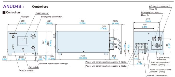
Note: The position and number of power unit communication connectors depend on the number of connected power units. See the chart on the right for the corresponding models. (Figure above shows an example of using 4 power units)
