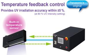
Generally, an increase in LED temperature reduces the UV irradiation output. However, the **UD40** series employs a Panasonic original head cooling mechanism to suppress temperature increases. Further, a temperature sensor is built into the head to constantly monitor and feed back temperature information. This has resulted in a superb UV irradiation stability within  $\pm 5$  % for output up to 80 %. This is ideal for high quality, precise adhesion applications.
