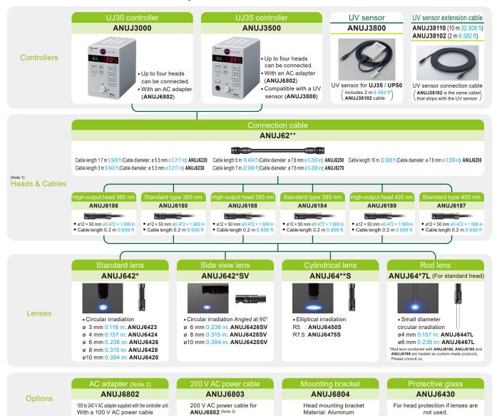
Notes: 1) The head does not come with a lens. 2) The ANUJ6602 AC adapter is supplied with the controller unit. The ANUJ6602 AC adapter is compatible with 100 to 240 V AC; however, the primary-side power cable is compatible with 100 V AC only. For use in a 200 V AC region, purchase the ANUJ6603 primary-side power cable (for 200 V AC) separately. 3) For China only. Primary-side A-type plug. (Since this product is not PSE Mark compliant, it cannot be connected directly to a lamp line in Japan.)
