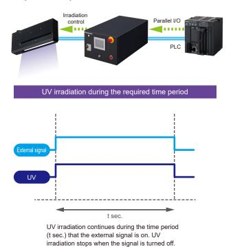
UV irradiation from the head can be controlled using a parallel signal from a PLC or other external device.
