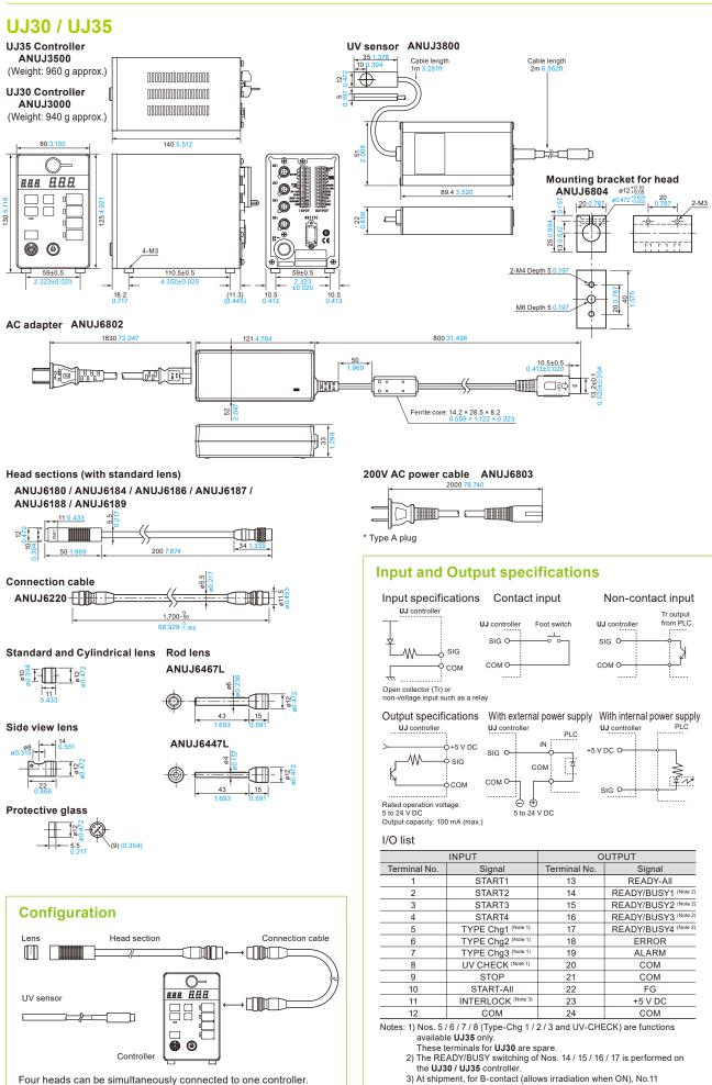
3) At shipment, for B-contact (allows irradiation when ON), No.11 (INTERLOCK) is connected to No.12 (COM) by a short-circuit line.
