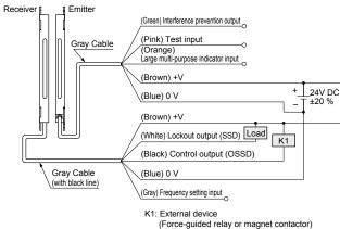
Wiring in case of using test input / large multi-purpose indicator / interference prevention functions
