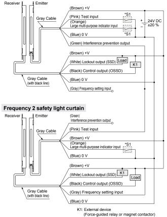
Note: If the large multi-purpose indicator input wiring (Orange) is connected to 0 V, the orange LED lights on. When they are disconnected, the orange LED lights off.
