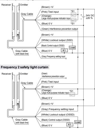
K1: External device (Force-guided relay or magnet contactor)
