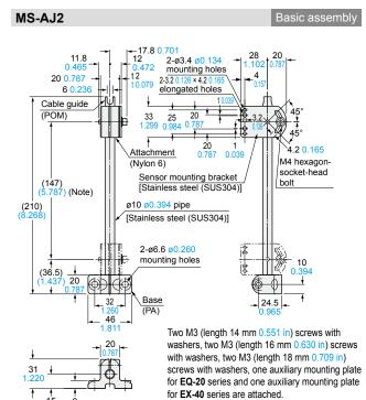
15 0.591 8 0.315 Note: The dimensions in the brackets indicate the adjustable range of the movable part.
