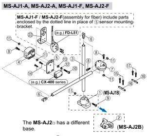
Note: Adjust the arm joint (⑦ in the figure) by loosening the M4 (length 12 mm 0.472 in) hexagon-socket-head bolts (⑧ in the figure) in two places. This way you can adjust the arm joint more smoothly.
