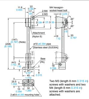
Note: The dimensions in the brackets indicate the adjustable range of the movable part.
