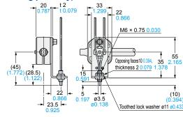
Note: The above diagram is in case of M6 threaded head fiber.
