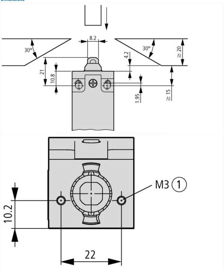
① screw-in depth max. 12 mm
