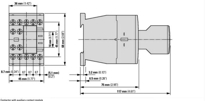
Contactor with auxiliary contact module
