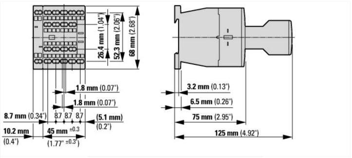
Contactor with auxiliary contact module
