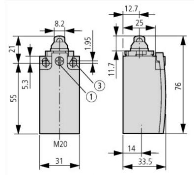
$\begin{array}{l} \textcircled{1}{1} \mbox{ Tightening torque of cover screws: 0.8 Nm \pm 0.2 Nm \\ \hline ($2$ only with LS (insulated version) \\ \hline ($3$ Fixing screws 2 x M4 $\ge 30$ \\ \hline M_A = 1.5 Nm \\ \end{array}$
