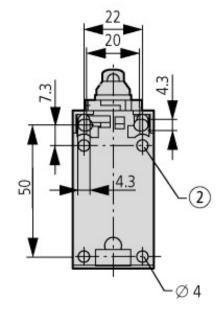
① Tightening torque Cover screw: 0.8 Nm ±0.2 Nm ② only with LS (insulated version) ③ Fixing screw 2 x M4 ≧ 30 M<sub>A</sub> = 1.5 Nm
