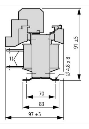
① Connection lugs ② With STI/STZ0.06 ... 0.16 ground connection at bottom
