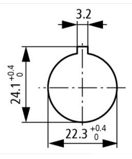
Door drilling dimensions Drilling dimensions: either 16.2 mm = without reduction  $\triangle$  RMQ16 or 22.3 mm = with reduction  $\triangle$  RMQ Titan
