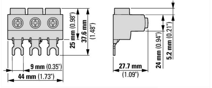
Overlapping mounting to extend the three-phase commoning link
