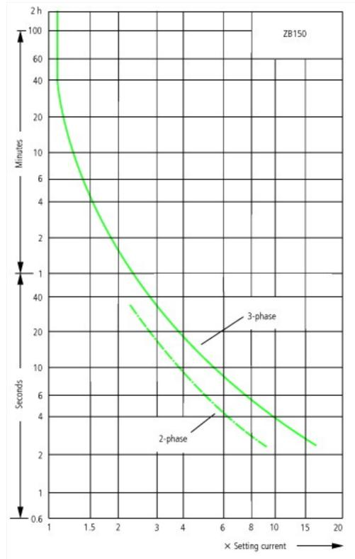
These tripping characteristics are mean values of the spread at 20 °C ambient temperature in a cold state. Tripping time depends on response current.
