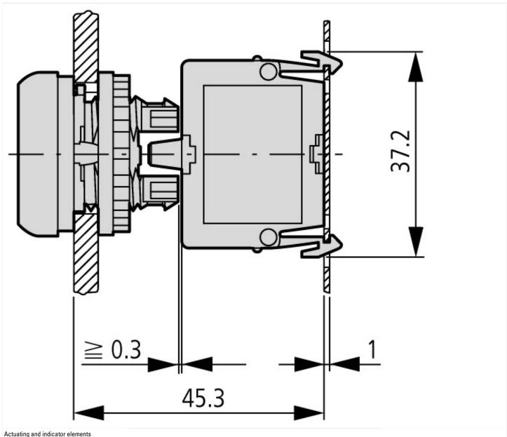
Actuating and indicator elements Base fixing
