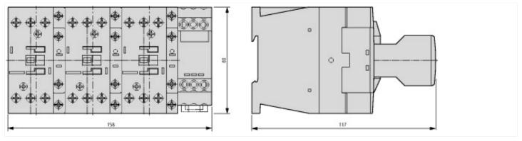
Basic unit with auxiliary contact module
