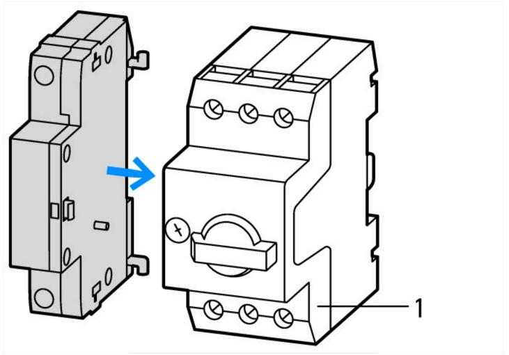
1: Motor-protective circuit-breakers
