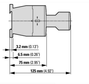
Contactor with auxiliary contact module
