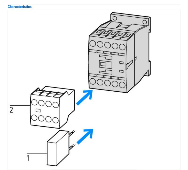
1: Suppressor 2: Auxiliary contact module
