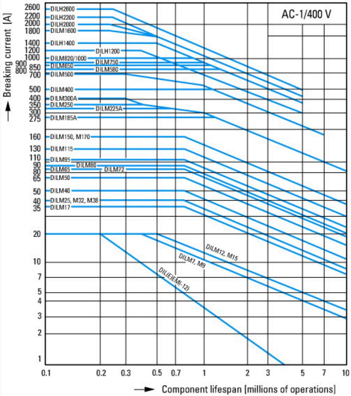
Switching conditions for 3 pole, non-motor loads
