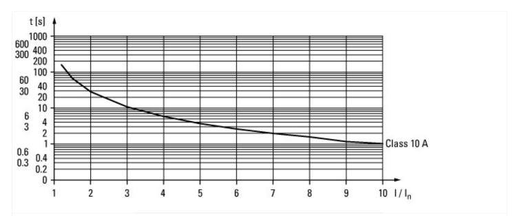
Tripping characteristics CLASS 10A set motor current > 4 A
