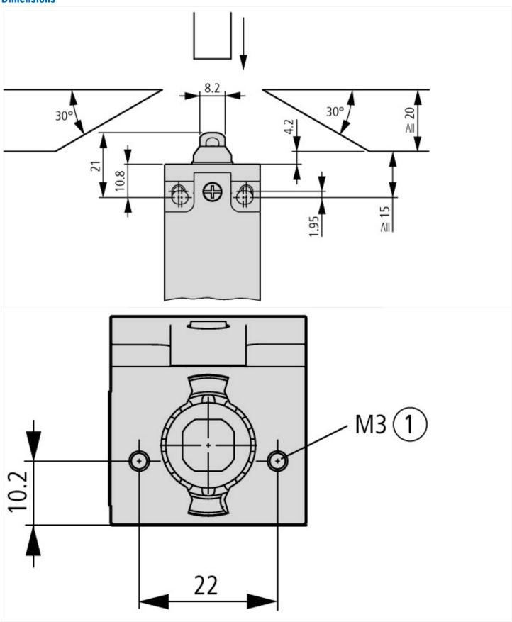
① screw-in depth max. 12 mm
