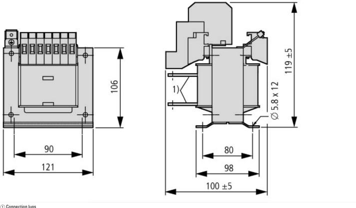
① Connection lugs ② With STI/STZ0.06 ... 0.16 ground connection at bottom
