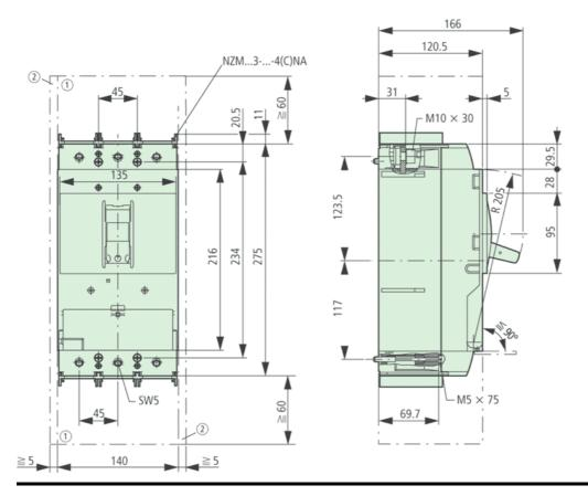
Arcing chamber, minimum clearing to neighbouring parts 60 mm Minimum clearance from adjacent parts 5 mm
