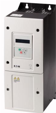
**Variable Frequency Drive, 3~/3~ 400 V, 39 A, 18.5 kW, Vector control, EMC-Filter, Brake-Chopper**
