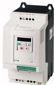
**Variable Frequency Drive, 3~/3~ 400 V, 24 A, 11 kW, Vector control, EMC-Filter, Brake-Chopper**
