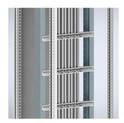
**Descrição:** Busbar supports up to 1600A to be mounted vertically behind the plug-in compartments. Rated short-time withstand current up to 35KA with rear supports and up to 50KA with rear and front supports. Mounts to the vertical profiles included in the rear cover plate for plugin sections MSSB.
