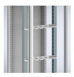
**Descrição:** Busbar supports up to 1600A to be mounted vertically behind the fixed compartments. Mounts to the vertical profiles MSFP. Rated short-time withstand current up to 35 kA with rear supports and up to 50 kA with rear and front supports.
