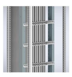
**Description:** Busbar supports up to 1600A to be mounted vertically behind the plug-in compartments. Rated short-time withstand current up to 35KA with rear supports and up to 50KA with rear and front supports. Mounts to the vertical profiles included in the rear cover plate for plugin sections MSSB.
