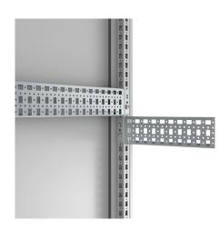
**Description:** Universal profile for both depth and width fitting on the 25 mm DIN hole pattern of the enclosure's frame or in combination with the CLPF and VB profiles. The 75 mm wide profile is equipped with three rows of holes of which one is turned 90°. This makes it possible to mount the CLPF profiles in both directions. The CLPK can be secured by the use of self tapping screws.
