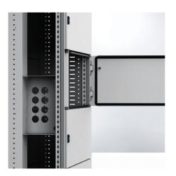
**Descripción:** Steel cable entrance box which lets us to build up a system with the terminations to functional unit separated from each other, meeting the Form 4. With the MSCE each functional unit (compartment) has its own integral glanding facility.
