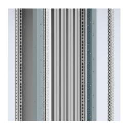
**Descripción:** Vertical busbar to build up the plug-in system. The MSBS bars are fixed in the MSVH supports with standard bolts, washers and nuts. The rated current can be increased up to  $2 \times 1400 \text{A}$  if the incoming connetion is in the middle.
